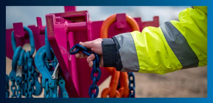
To protect against theft, a high-strength chain (grade 10; length approx. 1.5 m; eyelet thickness >= 10 mm) can be pulled through all suspension rings of the chain hangers and through the arms of the chain stand. The ends of the chains are then locked with a shackle lock (protection class 10).
