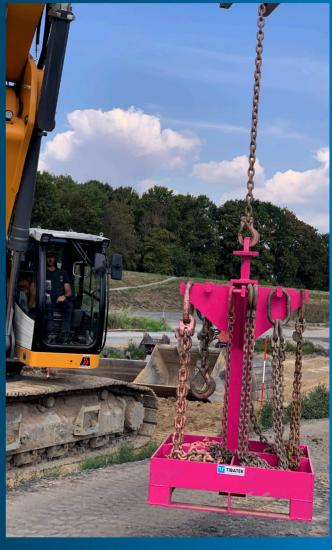
To move the chain stand, it can be attached to an excavator or crane. It can also be transported using a wheel loader + pallet fork or forklift truck.
